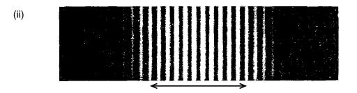
Since photograph is full-scale, by measuring using a ruler as shown: 13 fringe spacings = 4.5 cm [1] Hence fringe spacing  $\Delta x = 4.5/13 = 0.35$  cm = 3.5 x 10<sup>-3</sup> m [1]
