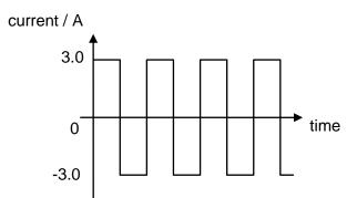
In order to obtain the same r.m.s. current as the waveform shown, a sinusoidal current of the same frequency should have a peak value of
