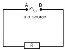
The voltage across AB varies sinusoidally with a peak voltage of 5.0 V as shown.
