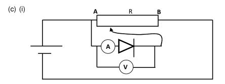
(ii) When the slider is at position A of Resistance R, the PD across the diode is zero and when the slider moves to position B, the PD across the diode reaches a value of 1.5 V.
